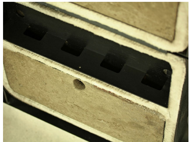
Special air ducts inside the doors allows pre-heating combustion air via natural air flow
