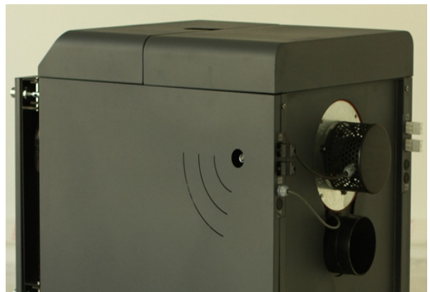
Induced draft fan keeps the system in constant vacuum eliminating the possibility of a smoke leakage to the ambient
