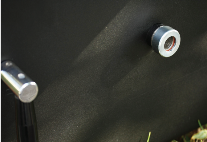
Observation Glass to Monitor Gasification Process
